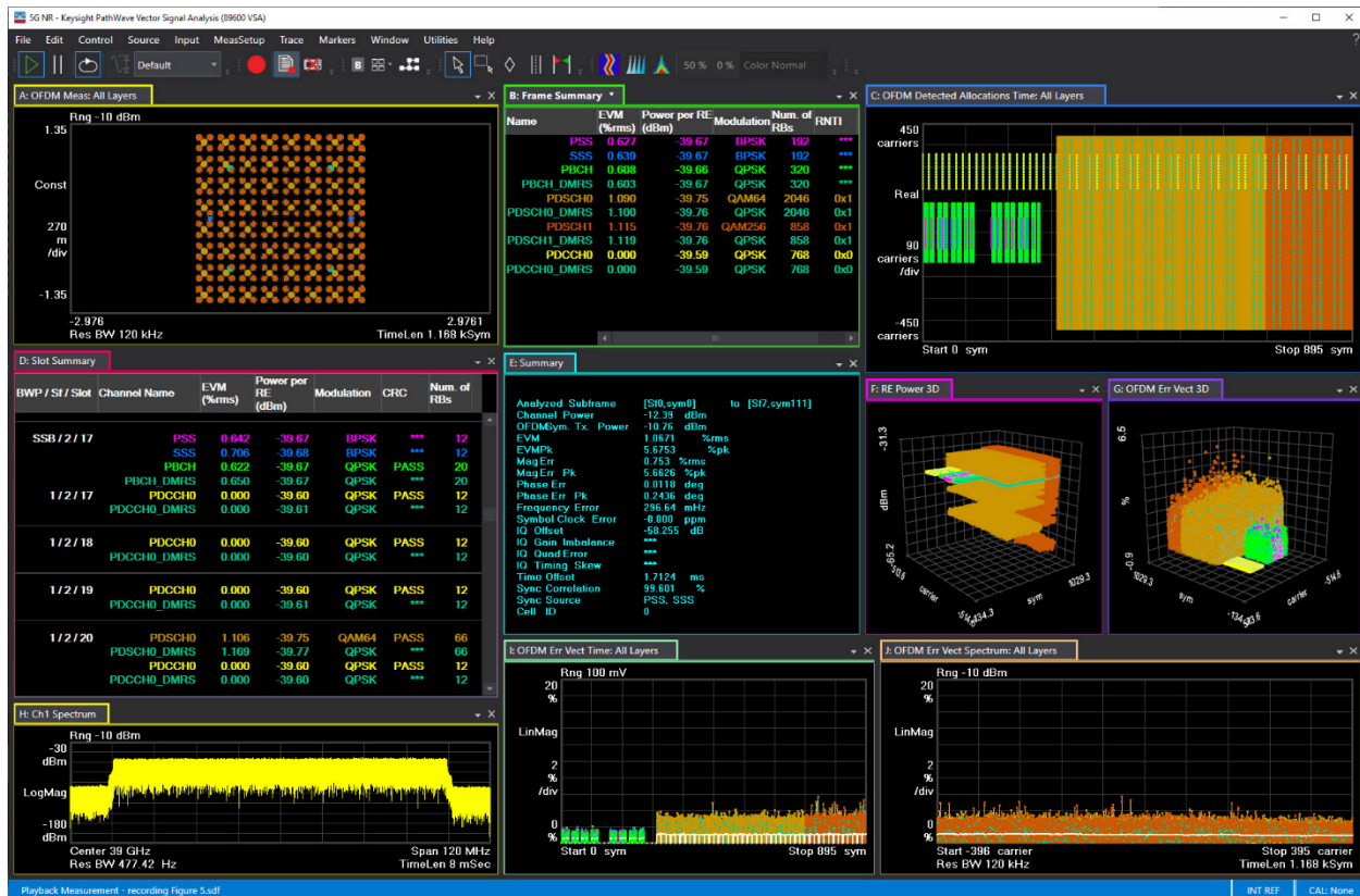
Figure 3. Example analysis of a downlink signal, at 39 GHz center frequency, with SS/PBCH, PDCCH and multiple PDSCHs.
