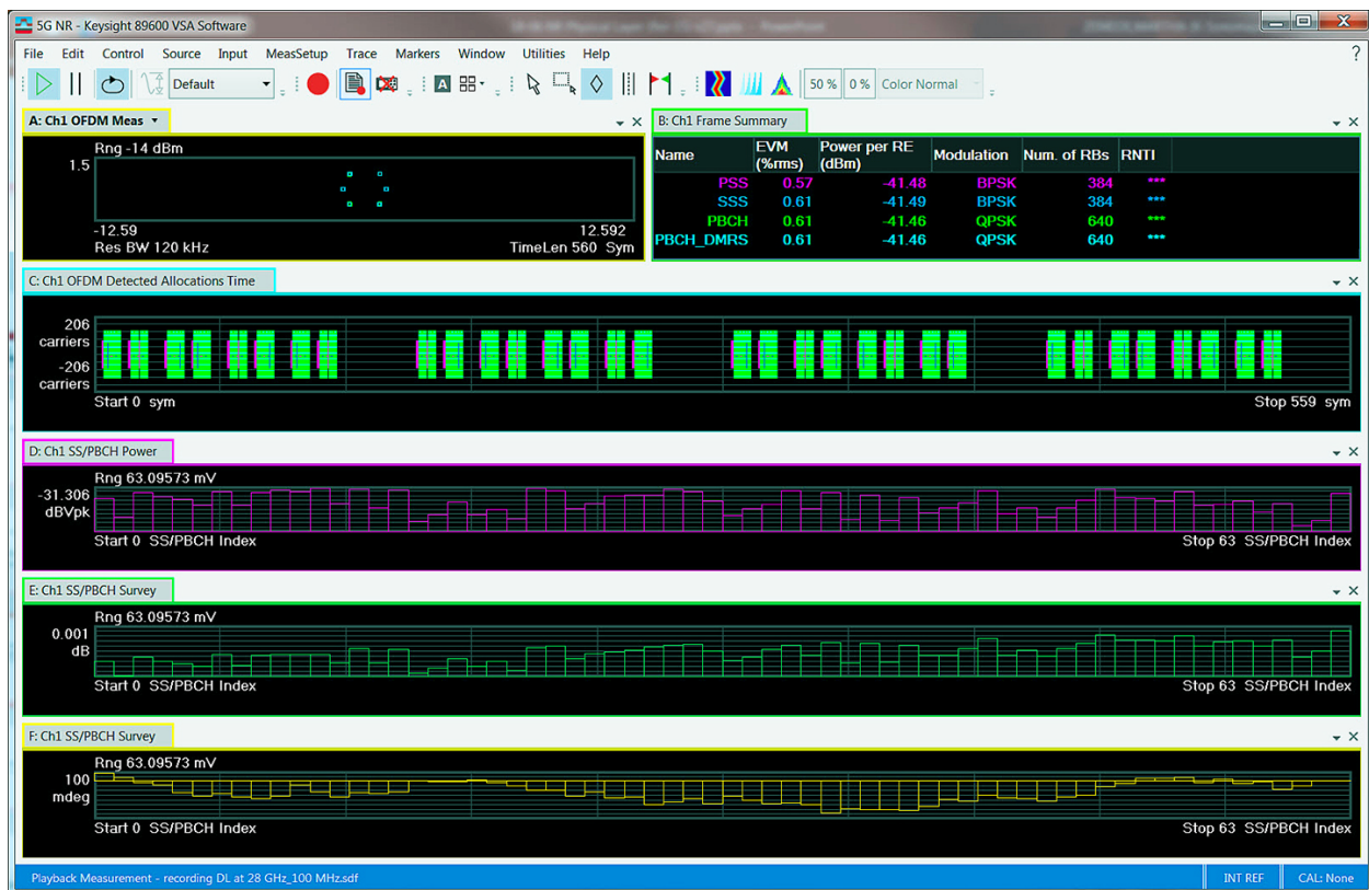
Figure 6. Example of SS/PBCH dedicated measurements to measure power and phase of each SS/PBCH active indices.
