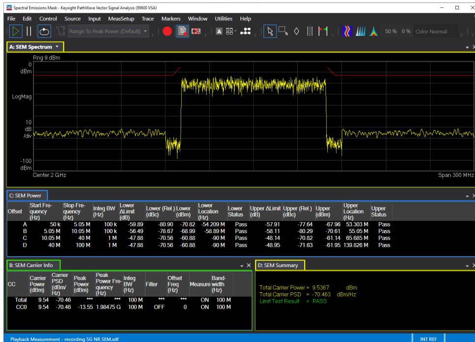
Figure 13. SEM measurement of a single carrier 5G NR signal
