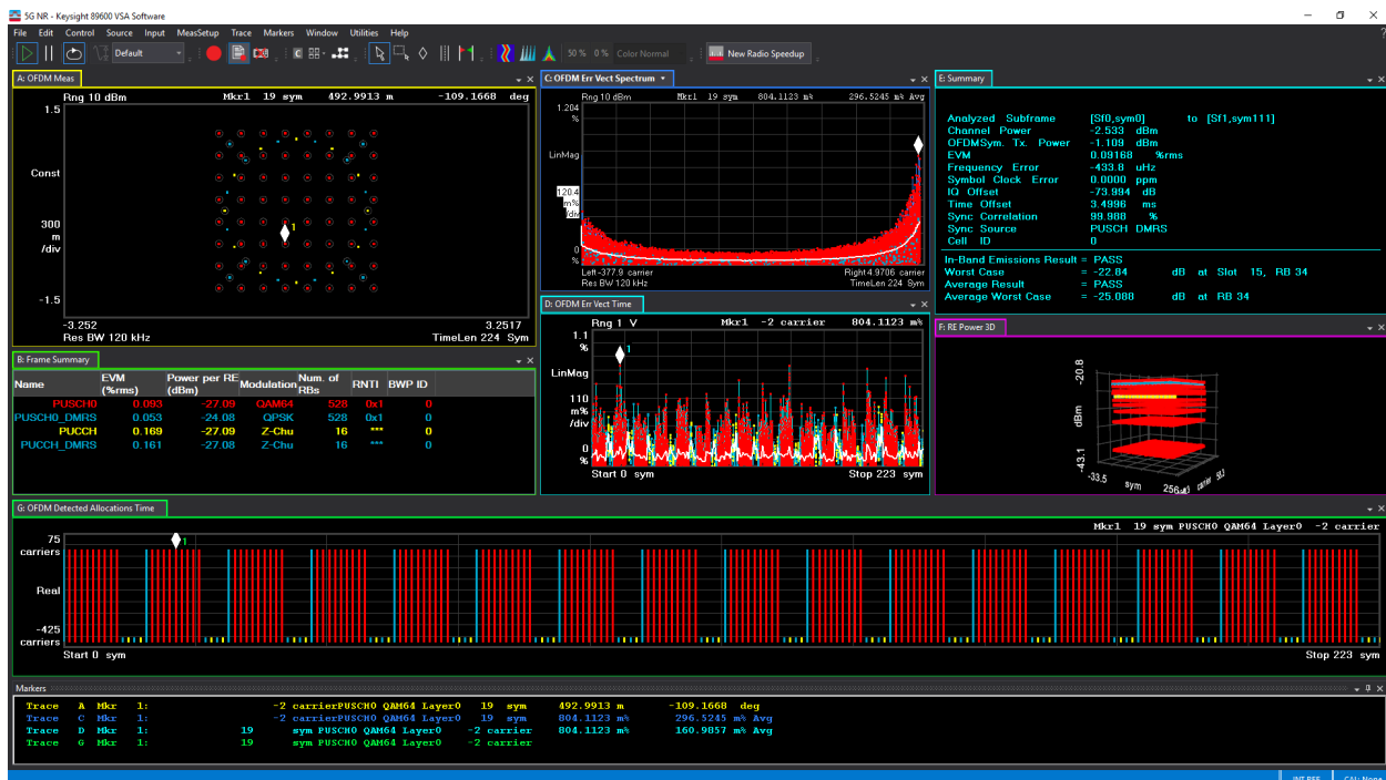
Figure 5. Example of coupled markers across multiple color-coded traces in different measurement domains.
