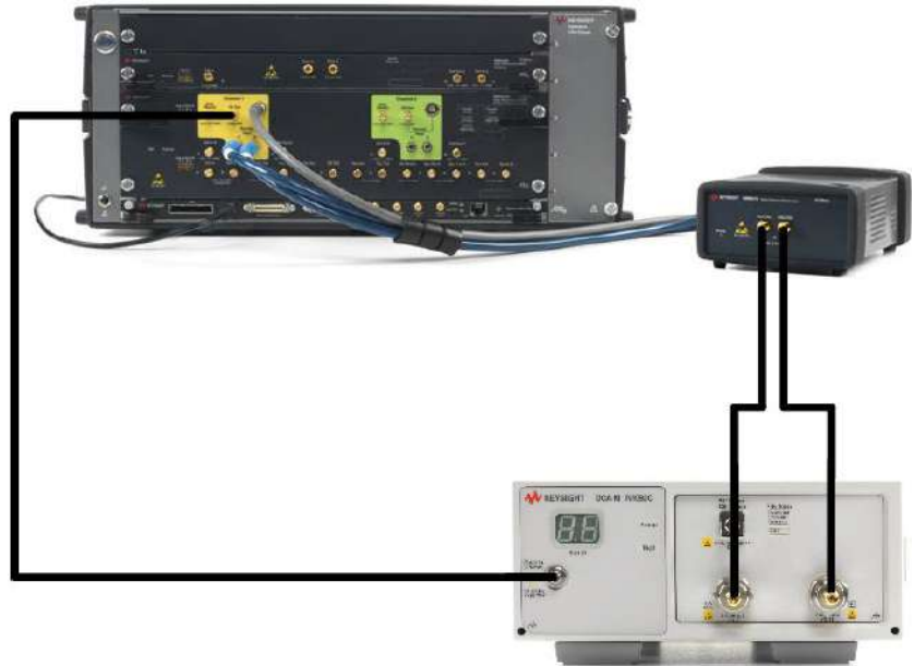
Connection among M8045A, M8057A/B and N1092C
