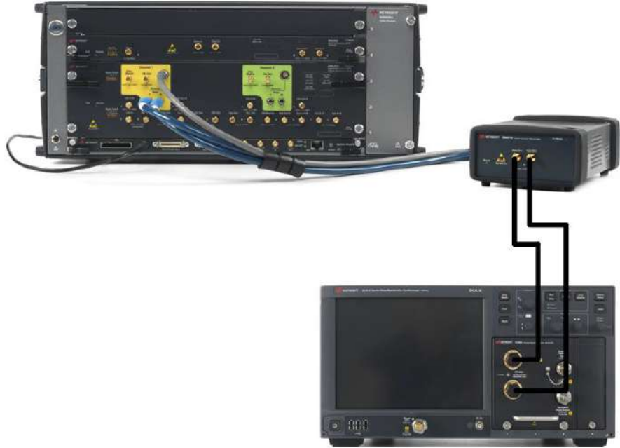
Connection among M8045A, M8057A/B and N1000A with N1060A
