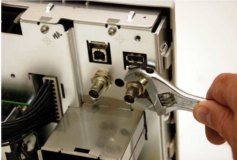
Figure 27 Removing the BNC nuts and washers
