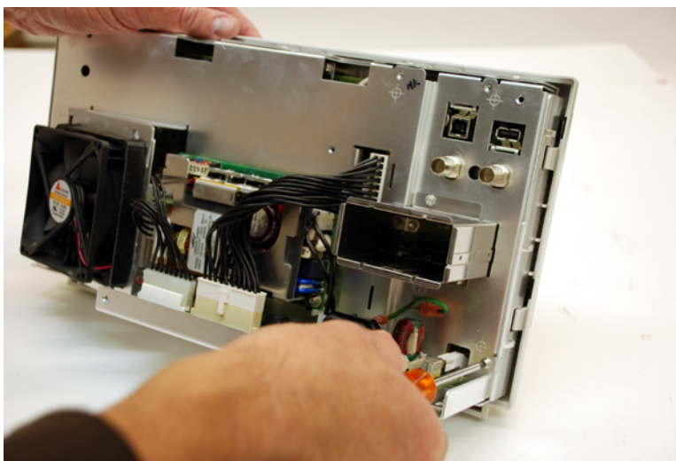
Figure 29 Removing the bottom right rear deck screw
