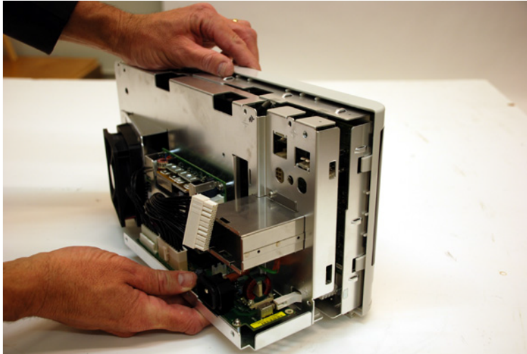
Figure 35 Separating the rear and front decks
