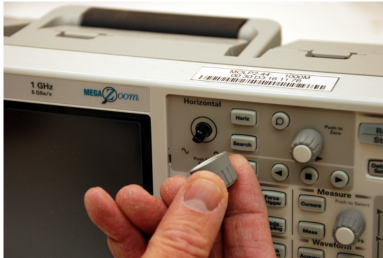
Figure 21 Removing the front panel knobs
