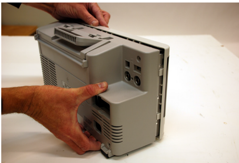
Figure 23 Removing bucket assembly
