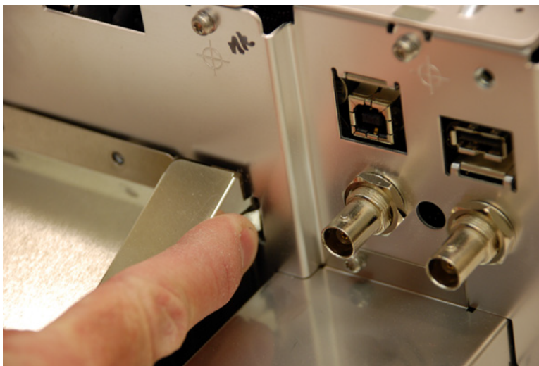
Figure 25 Unclipping the power supply shield right side
