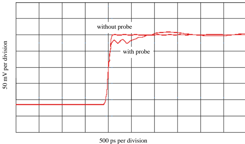
Figure 67 TDT measurement at receiver with and without probe load for 100 ps rise time
